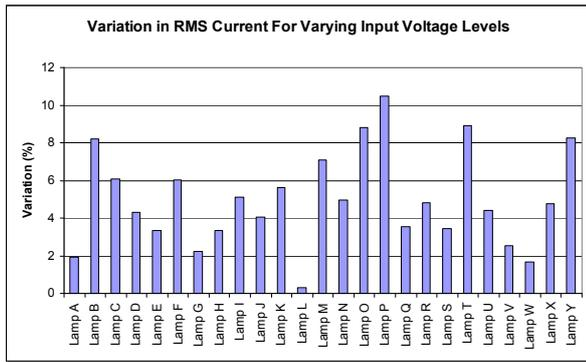
**Figure 6: Variation in the RMS Current Levels for Different Lamps for Varying Input Voltage Magnitudes**
