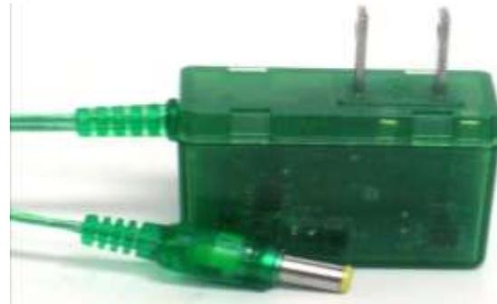
*Efficient 2 W External SMPS based on PI controller*
