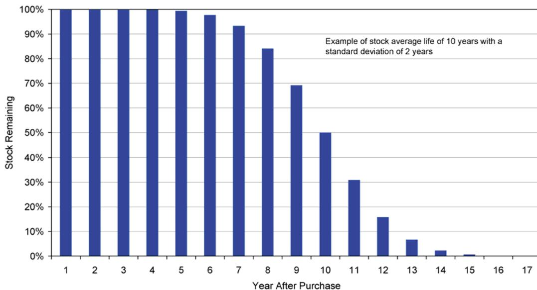
The stock model only uses the stock turnover function to estimate the change in average characteristics (attributes) of the stock by year (average mode power by year). The actual historical ownership and the projected ownership and stock should always be used to estimate the energy consumption of the product (not the implied stock numbers generated by the stock model). Of course, the ratio of actual stock to that projected by the model should be as close to unity as possible in all years.
