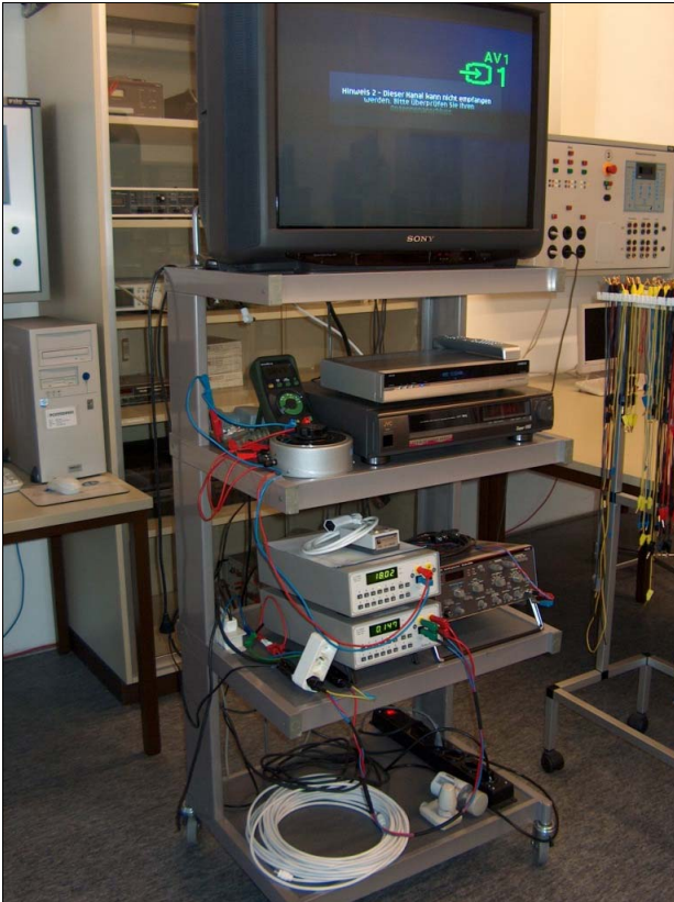
Photo 3: Measurements in the laboratory with Philips DSR9005 (DVB-S) set-top box
